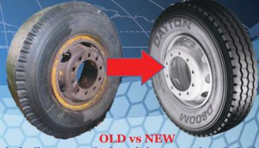
Old tubed split 15" & 16"wheel to tubeless tyre and 17.5" wheel Old tubed split 1000x20 wheel to tubeless tyre and 22.5" wheel
